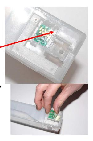
4. Reset the chip with a help of chip resetter by holding it the same as it shown in the picture. Keep it like this until the red flashing light will turn into green and then turns off.
