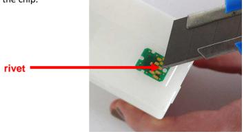
1. Remove the plastic nest which holds chip, together with chip from the refillable cartridge (using a small flathead screwdriver you need to lever the nest/plastic part which hold the chip)
